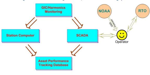
Figure A6-1: Functional diagram of GIC/Harmonics monitoring system
