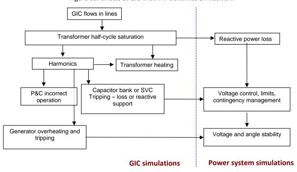
Figure 32: Effects of GIC in an HV transmission network
