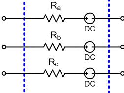
The quasi-DC voltage that is induced in each phase of a transmission line can be computed using Faraday's Law as defined in (1):
