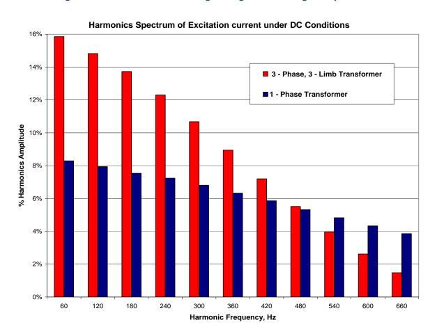
Figure 23: Harmonic content of magnetizing current during half-cycle saturation
