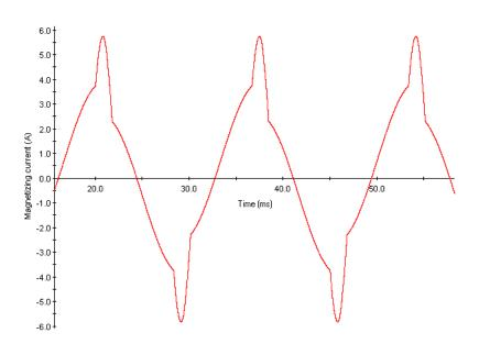
Figure 16: Transformer magnetizing current during saturation
