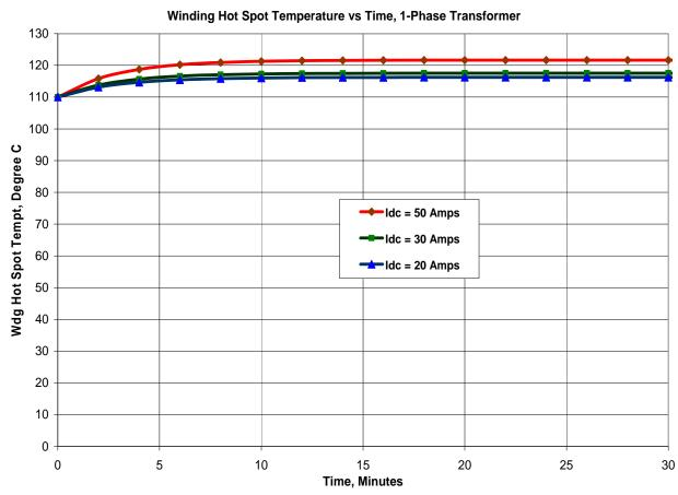
Figure 24: Winding hot spot temperatures for various values of DC current.
