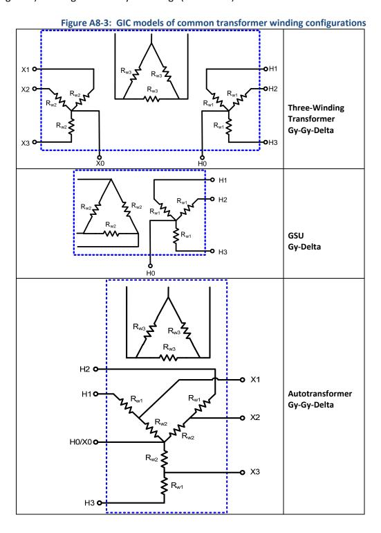
The resistance that is modeled is the DC winding resistance of the transformer. This information can be obtained from transformer test reports, but is not always available. The following assumptions can be used when test report data are unavailable.
