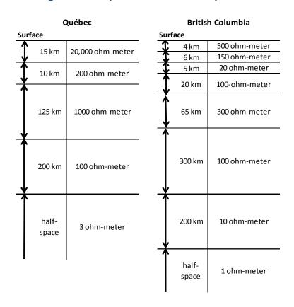
Figure 10: Examples of Earth conductivity models
