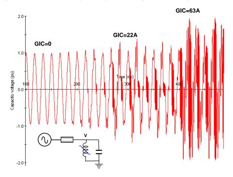
Figure 31: Illustrative example of capacitor voltage for increasing values of GIC
