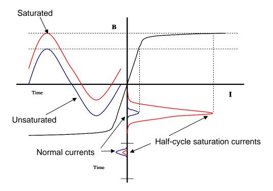
Figure 17: Relationship between flux and current with and without DC flux
