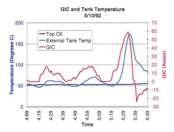
Figure 29: GIC and measured tank temperature<sup>82</sup>
