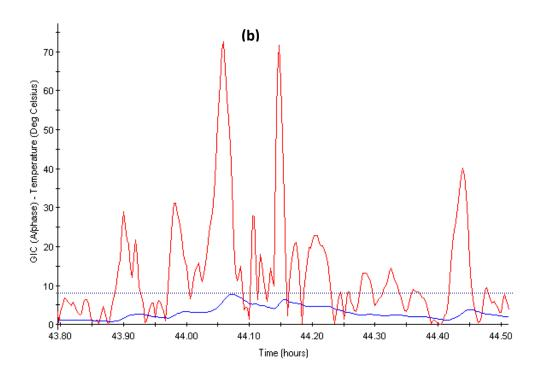
Figure 28: Tie plate temperature rise and GIC time series. Measured characteristics of a 400-MVA, 500/16.5-kV, single-phase transformer
