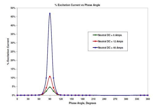
Figure 20: Magnetizing current pulse drawn from power grid under (AC+DC) excitation
