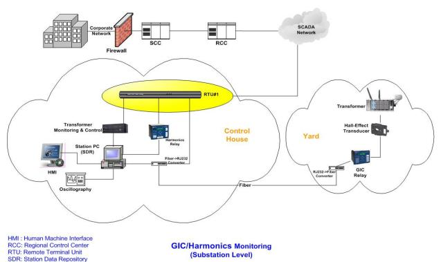
Figure A6-3: GIC/Harmonics Monitoring (GHM) System – substation level
